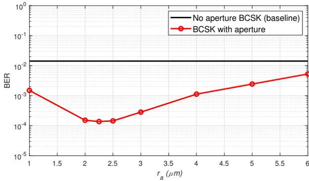
Fig. 2. BER vs.  $r_a$  curves for BCSK.  $t_s = 0.2$  s,  $d = 5$   $\mu\text{m}$ ,  $r_r = 5$   $\mu\text{m}$ ,  $d_a = 2$   $\mu\text{m}$ ,  $M = 1500$  molecules, diffusion coefficient  $D = 79.4$   $\mu\text{m}^2 \text{s}^{-1}$ .
