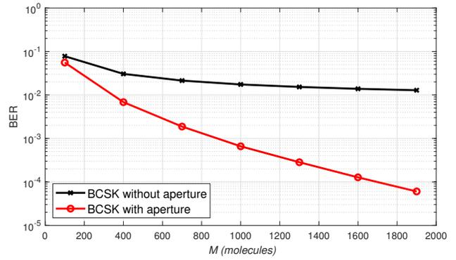
Fig. 3. BER vs.  $M$  curves for BCSK.  $t_s = 0.2$  s,  $d = 5$   $\mu\text{m}$ ,  $r_r = 5$   $\mu\text{m}$ ,  $d_a = 2$   $\mu\text{m}$ ,  $r_a = 2.25$   $\mu\text{m}$ ,  $D = 79.4$   $\mu\text{m}^2 \text{s}^{-1}$ .
